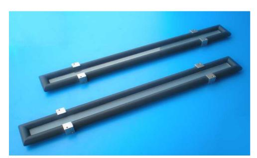
**ESCALON optical line scales** are artefacts to perform ISO 10360-7 conform performance verifications of video CMMs. All ESCALON artefacts feature the same two properties:
