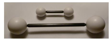
Our ball bars for the verification of laser scanners (VDI/VDE 2617-6) and fringe projectors (VDI/VDE 2634-1/2) have extremely dense mat ceramic balls. "Normal" industrial ceramic introduces systematic errors by "volume scattering" i.e. any pattern projected on the surface of a "normal" ceramic ball etc. is shifted in "downhill" direction and the measured diameter, position and form are affected.
