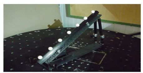
This is most disturbing when testing the performance of fringe projection systems. The here-used high density ceramics reduces this effect to practically not-disturbing levels. Very few competitors offer such artefacts.
