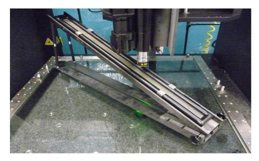
Unlike most line scales the **optical ESCALONs** can be fixed in different inclinations without changing their length, thanks to their neutral line assembly. The uncertainty of calibration can be performed better than  $U = 0.1 \mu m + 0.2 \mu m *L/m$ .
