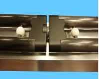
ESCALON ball bars can be optionally equipped with integrated high precision joints to assemble two or more ball bars so that they form together one entirely calibrated ball bar. No stitching is needed as we work with one big ball bar.
