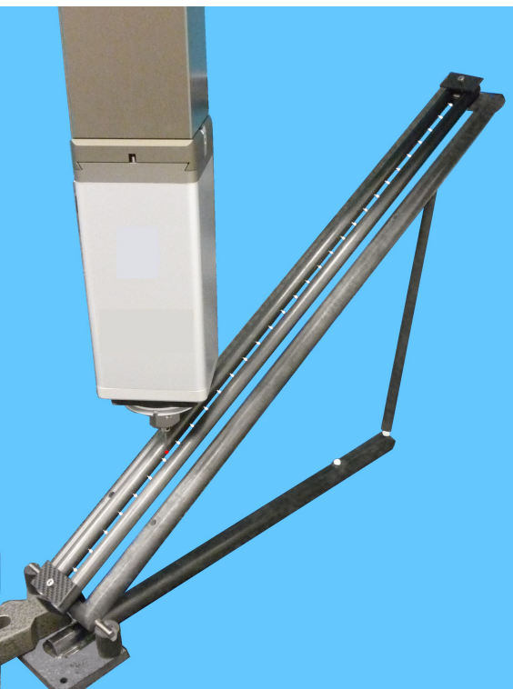
CMM checked with 1 m "Miniatur" ESCALON
